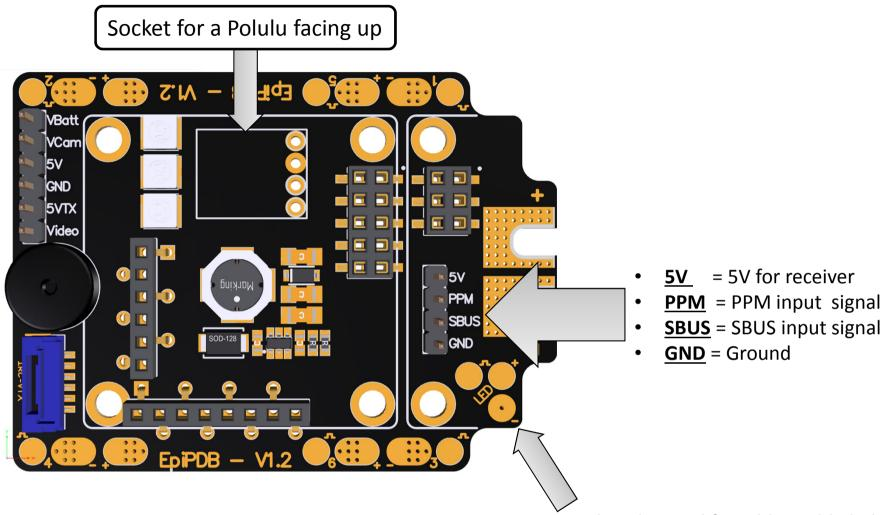
Pads to be used for addressable leds
